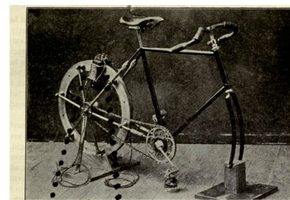
FIG. 4.—The Bicycle Ergometer. The rear wheel of a bicycle is replaced by a copper disk which can rotate in the field of a magnet. The strength of the magnet can be varied by the quantity of electricity passing through the field coils. The principle is that of the electric brake.
