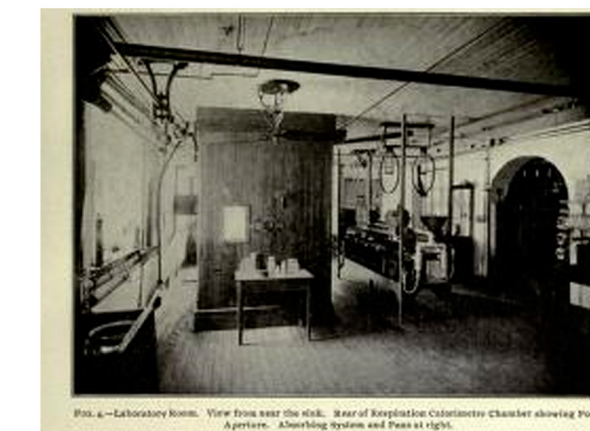
FIG. 4.—Laboratory Room. View from east side. Rear of Respiration Chamber showing Food Apertures, Absorbing System and Pass at right.
